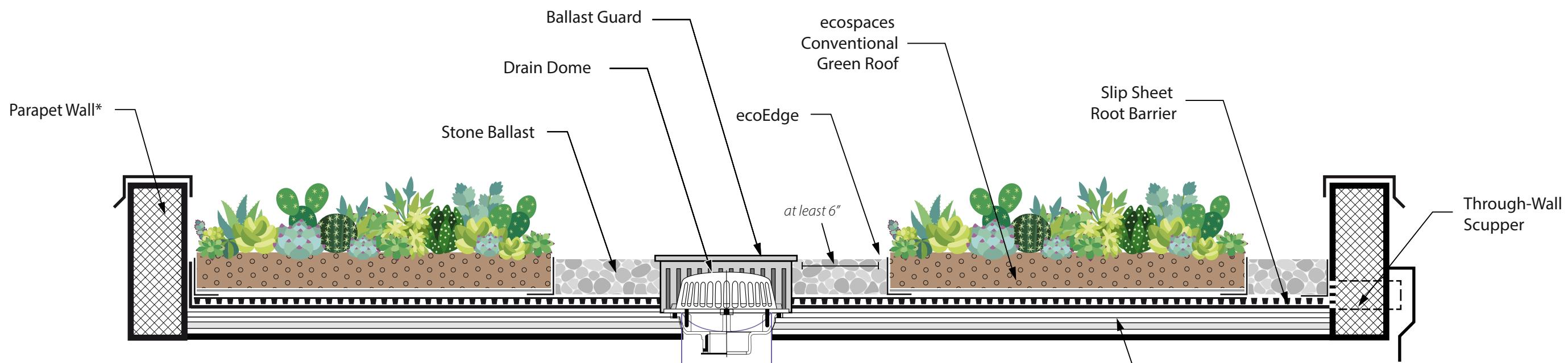
\* In most cases, ecospaces built-in-place green roof system can extend directly to the parapet wall; or a stone ballast border can be used between the ecoEdge and the parapet wall.
